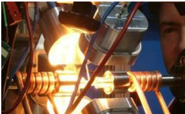
In-situ neutron experiments at high temperatures and load.
