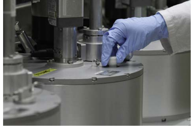
For NAA, samples are sent into the irradiation positions near the reactor core using the pneumatic rabbit irradiation system.
