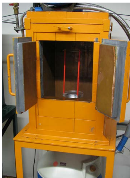
Fig. 2: A high-purity germanium detector with shielded counting chamber.
